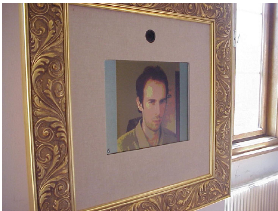
15 seconds of fame: and LCD computer monitor is framed like a painting. The round opening above the picture is for the digital camera lens.
